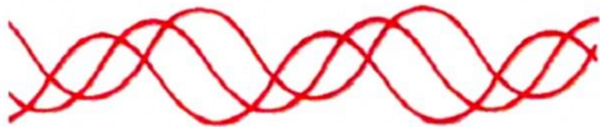
LED: one color (monochromatic) and waves not in phase (non-coherent)
